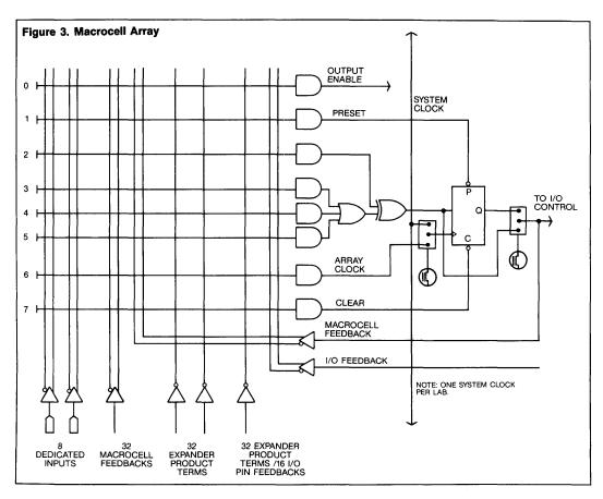
logic implementation and the remainder for control logic. These 3 terms are OR'ed together forming a Sum-Of-Product result that is then XOR'ed with a single product term. This single term controls logic inversion. By setting this inversion term to logic true or "1", the Sum-Of-Product result is always complemented providing active low operation.
