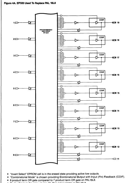
Pin feedback to the array at pins 12, 19 is not available in PAL16L8.
