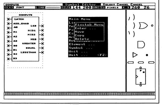
Entry, State Machine, or Boolean descriptions. This provides a wide range of flexibility for the designer, allowing Boolean Equations to be mixed with State Machine entry in a hierarchical schematic. The created function may now be entered into the higher level schematic, or any schematic in subsequent designs.
