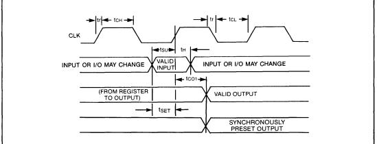
Notes: tr & tr < 6ns; tcL & tcH measured at 0.3V and 2.7V; all other timings at 1.5V; Input voltage levels at 0V and 3V
