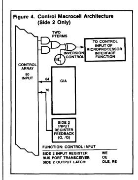
The Microprocessor Interface Functions shown in Figure 5 provide access to the different configurations for the input registers, output latches and bus port transceiver. Definitions for each function are given in Table 1.
