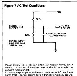
Large amplitude, fast ground current transients normally occur as the device outputs discharge the load capacitances. These transients flowing through the parasitic inductance between the device ground pin and the test system ground can create significant reductions in observable input noise immunity.
