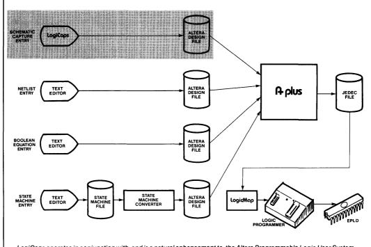
LogiCaps operates in conjunction with, and is a natural enhancement to, the Altera Programmable Logic User System (A+PLUS). It provides a complete path from the engineer's design concept to a programmed EPLD.
