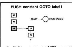
The PUSH constant to stack GOTO command will push the value constant onto the Stack and jump to label1. In the example, address 44 has the command 'PUSH 34D GOTO label1' where label1 is located at address 73. The decimal value 34 is pushed onto the Stack and the next state comes from address 73. The default for label1 is the next instruction in the 'ASM file.
