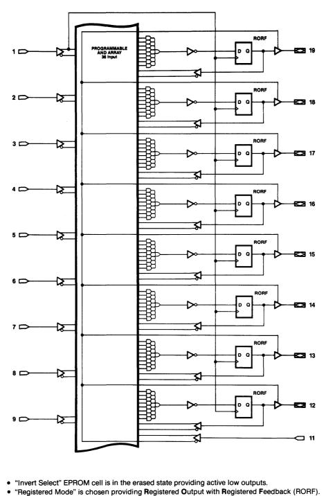
• Complement of pin 11 is used as common OE term for all 8 output pins.
