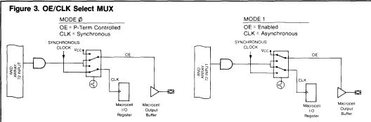
The register is clocked by the synchronous clock signal which is common to 11 other Macrocells. The output is enabled by the logic from the product term. The output is permanently enabled and the register is clocked via the product term. This allows for gated clocks that may be generated from elsewhere in the EP910.
