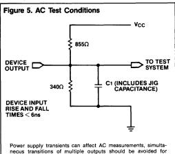
neous transitions of multiple outputs should be avoided for accurate measurement. Do not attempt to perform threshold tests under AC conditions. Large amplitude, fast ground current transients normally occur as the device outputs discharge the load capacitances. These transients flowing through the parasitic inductance between the device ground pin and the test system ground can create significant reductions in observable input noise immunity.
